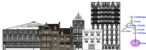
Figure 10: The user can directly design buildings with a user-friendly graph-based paradigm. From an initial building, the Raccollet House (colored in the front), we have easily created all the other buildings in this Figure.
