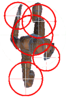
Figure 5: Collision model of 5 cylinders around the head, the left and right hands, and the left and right foot.
