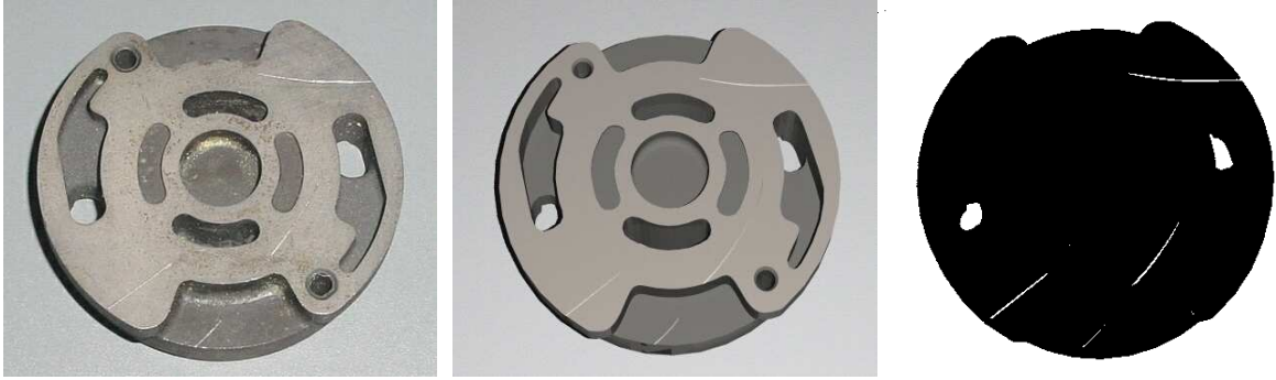
Figure 4.7: Left: a real scratched metallic part. Middle: its corresponding synthetic image. Right: detection of the scratches.
