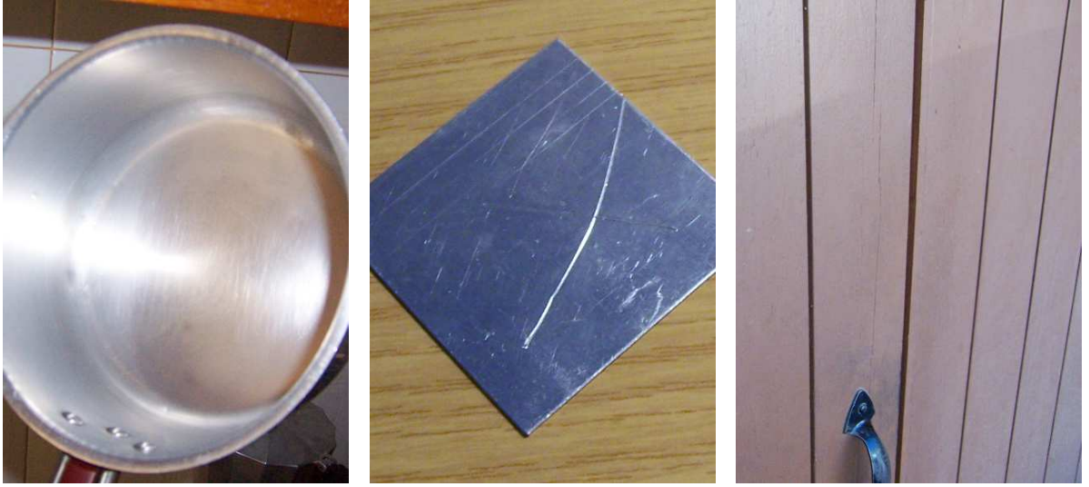
Figure 1.1: Pictures of real surfaces exhibiting scratches or grooves. From left to right: a polished pan with lots of micro-scratches, a metallic plate with isolated scratches, and a door with big grooves between the wooden planks.
